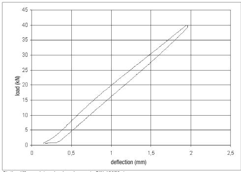
Static stiffness determined analogous to DIN 45673-1.
